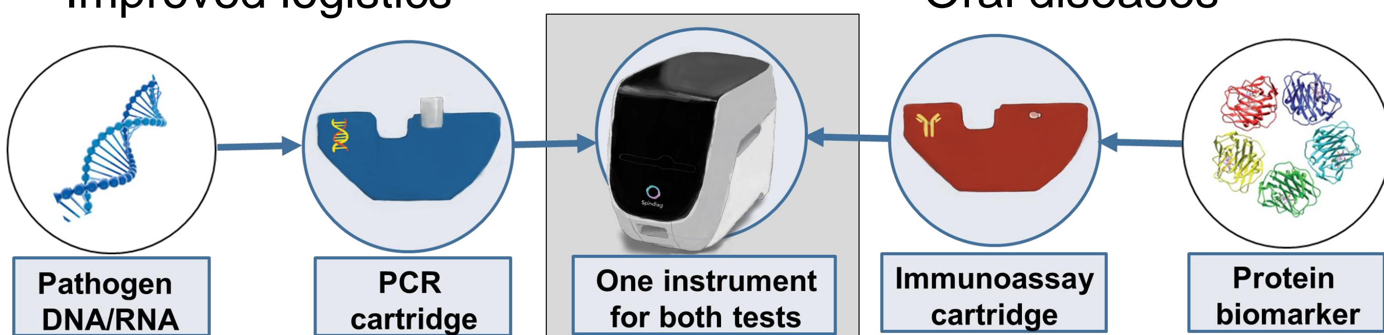
Fig. 3: BFPD-IA enables PCR & Immunoassay on the same instrument
